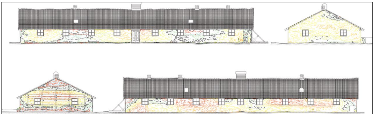
Fig. 5. Scan image of the gable wall of barrack B-123 based on scans provided by Geotronics Poland; source: S. Karczmarczyk et al., op. cit., by R. Paruch.
