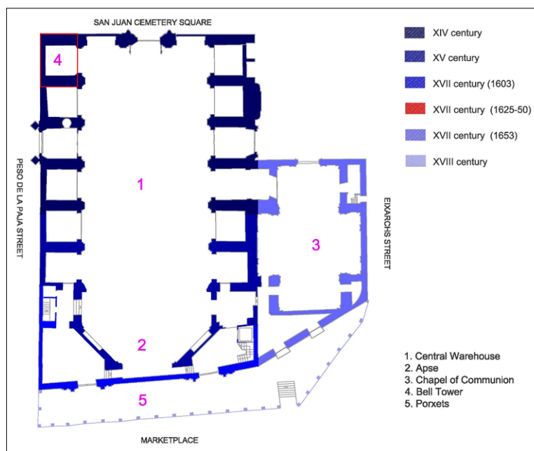
Fig. 1. Santos Juanes Church, floor plan with wall layers in chronological order (upper legend); and descriptions of distinctive structural elements (bottom legend); by the authors.
