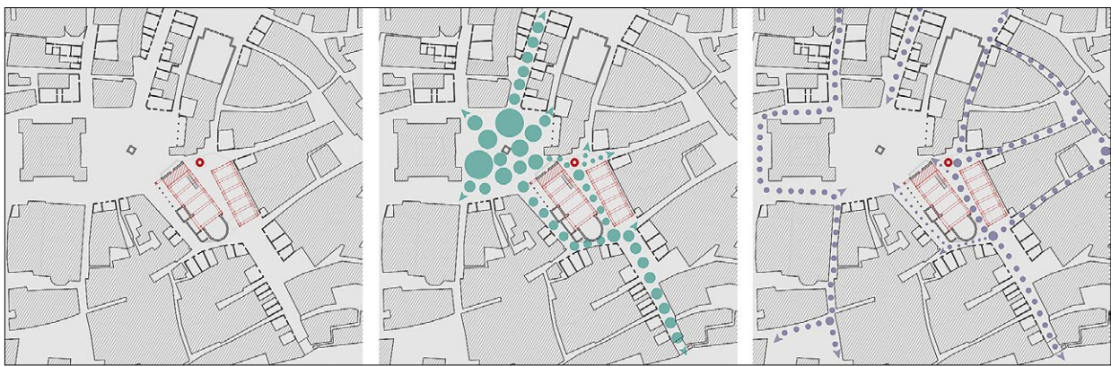
Fig. 7. The area of St. Benedict Square in Norcia, Italy, after the 2016 AVN seismic sequence: modular and reusable system scenario; from the left: a) urban tissue, b) walkability, c) accessibility for vehicles; by A. Rogulska
